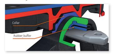
The K-bearing moves especially easy and it is torsion-proof and maintenance-free. It protects the chassis due to its longitudinal elasticity (lateral movement).
