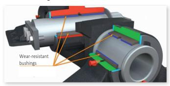
The cardanic bearing is designed to allow roll between tractor and semi-trailer under off-road conditions. Due to the high strains it is designed as pivot bearing with wear-resistant bearing bushings. The lateral suspension must be disabled for on-road use.
