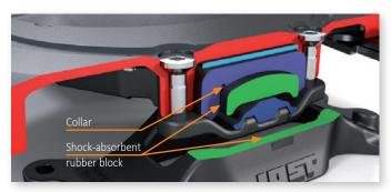
The new hybrid bearing combines the advantages of the rubber and the slide bearing. The rubber cushions are shock-absorbent and maintenance-free. Thanks to the plastic collars it protects the chassis due to its longitudinal elasticity (lateral movement).
