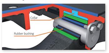
The pivot bearing allows low mounting heights and is maintenance-free in the "E" version. It is particularly suitable for use in sliding and dual height fifth wheel systems.
