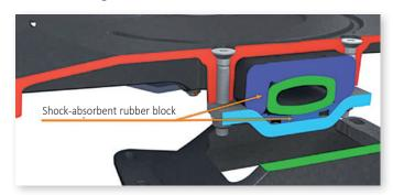
Fifth wheel couplings with rubber mountings are particularly suitable for poor quality road surfaces. The rubber cushions are shock-absorbent and maintenance-free.
