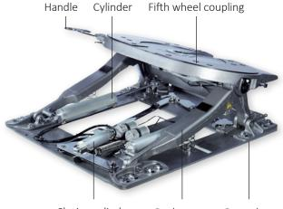
Closing cylinder Rocker arm Base plate
